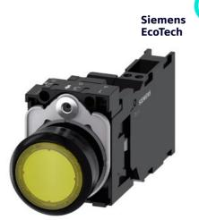
Illuminated pushbutton, 22 mm, round, plastic, yellow, pushbutton, flat, momentary contact type, with holder, 1 NO+1 NC, LED module with integrated LED 110 V AC, spring-type terminal, with laser labeling, upper case and lower case, always upper case at beginning of line
