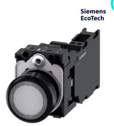
Illuminated pushbutton, 22 mm, round, plastic, clear, pushbutton, flat, momentary contact type, with holder, 1 NO+1 NC, LED module with integrated LED 24 V AC/DC, spring-type terminal, with laser labeling, upper case and lower case, Always upper case at the beginning of the word
