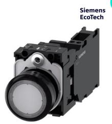
Illuminated pushbutton, 22 mm, round, plastic, clear, pushbutton, flat, momentary contact type, with holder, 1 NO+1 NC, LED module with integrated LED 24 V AC/DC, spring-type terminal, with laser labeling, upper case
