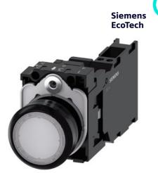
Illuminated pushbutton, 22 mm, round, plastic, white, pushbutton, flat, momentary contact type, with holder, 1 NO+1 NC, LED module with integrated LED 24 V AC/DC, spring-type terminal, with laser labeling, symbol number according to, ISO 7000 or IEC 60417
