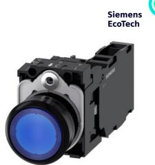
Illuminated pushbutton, 22 mm, round, plastic, blue, pushbutton, flat, momentary contact type, with holder, 1 NO+1 NC, LED module with integrated LED 24 V AC/DC, screw terminal, with laser labeling, lower case
