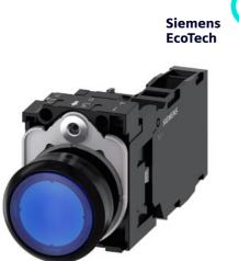
Illuminated pushbutton, 22 mm, round, plastic, blue, pushbutton, flat, momentary contact type, with holder, 1 NO+1 NC, LED module with integrated LED 24 V AC/DC, screw terminal, with laser labeling, upper case
