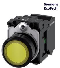
Illuminated pushbutton, 22 mm, round, plastic, yellow, pushbutton, flat, momentary contact type, with holder, 1NO, LED module with integrated LED 24 V AC/DC, spring-type terminal, with laser labeling, inscription or symbol Customer-specific selection with SIRIUS ACT configurator (CIN)
