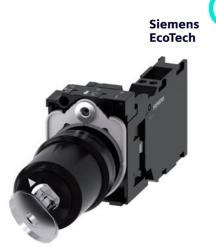
key-operated switch Siemens, 22 mm, round, plastic, lock number SSG10, with 2 keys, 2 switch positions O-I, latching, 10:30h/13:30h, key removal O+I, with holder, 1 NO+1 NC, spring-loaded terminal, with laser labeling, upper case and lower case, always upper case at beginning of line
