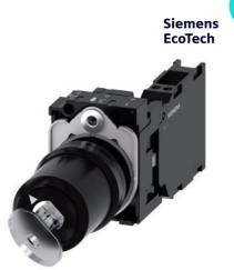
key-operated switch Siemens, 22 mm, round, plastic, lock number SSG10, with 2 keys, 2 switch positions O-I, latching, 10:30h/13:30h, key removal O+I, with holder, 1 NO+1 NC, spring-loaded terminal, Z=20-unit packaging
