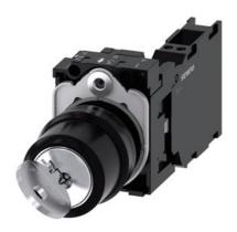
RONIS key-operated switch, 22 mm, round, plastic, Lock No. SB30, with 2 keys, 2 switch positions O-I, latching, 10:30/1:30 o'clock, key removal O+I, with holder, 1NO+1NC, spring-type terminals, possible special locks: SB31, 421, 455, Z=20-unit packaging
