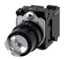
RONIS key-operated switch, 22 mm, round, plastic, lock number SB30, with 2 keys, 2 switch positions O-I, latching, 10:30h/13:30h, key removal O+I, with holder, 1 NO, spring-type terminal, possible special locks: SB31, 421, 455, with laser labeling, inscription or symbol Customer-specific selection with SIRIUS ACT configurator (CIN)
