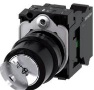
RONIS key-operated switch, 22 mm, round, plastic, lock number SB30, with 2 keys, 2 switch positions O-I, latching, 10:30h/13:30h, key removal O+I, with holder, 1 NO, spring-type terminal, possible special locks: SB31, 421, 455, with laser labeling, upper case and lower case, always upper case at the beginning of the word
