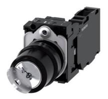
RONIS key-operated switch, 22 mm, round, plastic, lock number SB30, with 2 keys, 2 switch positions O-I, latching, 10:30h/13:30h, key removal O+I, with holder, 1 NO+1 NC, screw terminal, possible special locks: SB31, 421, 455, with laser labeling, upper case and lower case, always upper case at the beginning of the word
