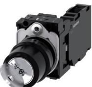
RONIS key-operated switch, 22 mm, round, plastic, lock number SB30, with 2 keys, 2 switch positions O-I, latching, 10:30h/13:30h, key removal O+I, with holder, 1 NO+1 NC, screw terminal, possible special locks: SB31, 421, 455, with laser labeling, lower case
