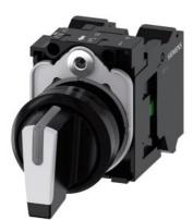
Selector switch, illuminable, 22 mm, round, plastic, white, selector switch, short, 3 switch positions I>O<II, momentary contact type, 10:30h/12h/13:30h, with holder, 1 NO, 1 NO, spring-type terminal, with laser labeling, upper case
