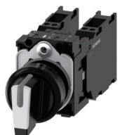
Selector switch, illuminable, 22 mm, round, plastic, white, selector switch, short, 3 switch positions |>O<|I|, momentary contact type, 10:30h/12h/13:30h, with holder, 2 x 1 NO+1 NC, spring-type terminal, with laser labeling, upper case and lower case, always upper case at beginning of line
