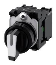
Selector switch, illuminable, 22 mm, round, plastic, white, selector switch, short, 3 switch positions I>O<II, momentary contact type, 10:30h/12h/13:30h, with holder, 1 NO, 1 NO, screw terminal, with laser labeling, upper case and lower case, always upper case at the beginning of the word
