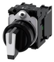
Selector switch, illuminable, 22 mm, round, plastic, white, selector switch, short, 3 switch positions I>O<II, momentary contact type, 10:30h/12h/13:30h, with holder, 1 NO, 1 NO, screw terminal, with laser labeling, lower case
