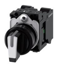
Selector switch, illuminable, 22 mm, round, plastic, white, selector switch, short, 3 switch positions I-O-II, latching, 10:30h/12h/13:30h, with holder, 1 NO, 1 NO, spring-type terminal, with laser labeling, upper case and lower case, always upper case at beginning of line
