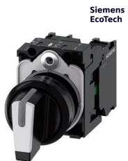
Selector switch, illuminable, 22 mm, round, plastic, white, selector switch, short, 3 switch positions I-O-II, latching, 10:30h/12h/13:30h, with holder, 1 NO, 1 NO, screw terminal, with laser labeling, lower case
