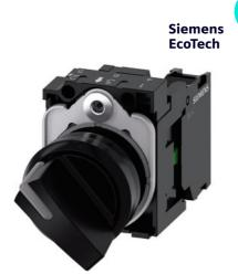
Selector switch, Illuminable 22 mm, round, plastic, black, knob, short 2 switch positions O-I, latching, 10:30h/13:30h, with holder, 1 NO, screw terminal
