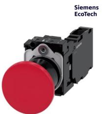
Mushroom pushbutton, 22 mm, round, plastic, red, 40mm, latching, pull-to-unlatch mechanism, with holder, 1 NO+1 NC, screw terminal, with laser labeling, upper case and lower case, always upper case at beginning of line
