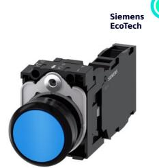
Pushbutton, 22 mm, round, plastic, blue, pushbutton, flat, momentary contact type, with holder 1 NO+1 NC, screw terminal, with laser labeling, upper case and lower case, always upper case at beginning of line
