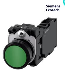
Pushbutton, 22 mm, round, plastic, green, pushbutton, flat, momentary contact type, with holder 1 NO+1 NC, screw terminal,
