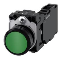
Pushbutton, 22 mm, round, plastic, green, pushbutton, flat, momentary contact type, with holder 1 NO+1 NC, screw terminal, Z=20-unit packaging
