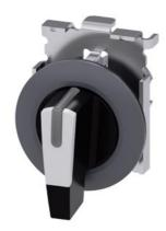
Selector switch, illuminable, 30 mm, round, Metal, matte, white, selector switch, long, front ring for flush installation, 3 switch positions I>O<II, momentary contact type, actuating angle  $2x45^{\circ}$ , 10:30h/12h/13:30h, with laser labeling, lower case
