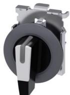
Selector switch, illuminable, 30 mm, round, Metal, matte, white, selector switch, long, front ring for flush installation, 3 switch positions I>O<II, momentary contact type, actuating angle 2x45°, 10:30h/12h/13:30h, with laser labeling, upper case
