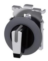
Selector switch, illuminable, 30 mm, round, Metal, matte, white, selector switch, short, front ring for flush installation, 3 switch positions I-O<II, left latching, right momentary contact type, actuating angle 2x45°, 10:30h/12h/13:30h
