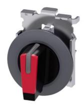
Selector switch, illuminable, 30 mm, round, metal, matte, red, selector switch, short, front ring for flush installation, 3 switch positions I-O-II, latching, actuating angle  $2x45^{\circ}$ , 10:30h/12h/13:30h
