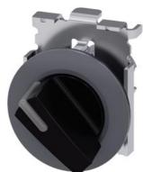
Illuminable selector switch, 30 mm, round, Metal matte, black, Selector switch short, front ring for flush installation, latching, actuating angle 90°, 10:30h/13:30h
