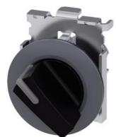
Illuminable selector switch, 30 mm, round, Metal matte, black, Selector switch short, front ring for flush installation, momentary contact type, Actuating angle 45°, 10:30h/12h
