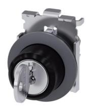
RONIS key-operated switch, 30 mm, round, metal, matte, front ring for flush installation, lock number SB30, with 2 keys, 3 switch positions I-O-II, latching, actuating angle 2x45°, 10:30h/12h/13:30h, Key removal I+O+II, possible special locks: SB31, 421, 455
