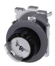
RONIS key-operated switch, 30 mm, round, metal, matte, front ring for flush installation, lock number SB30, with 2 keys, 2 switch positions O<1, momentary contact type, Actuating angle 45°, 10:30h/12h, key removal O, possible special locks: SB31, 421, 455
