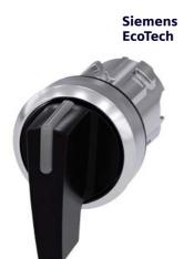
Illuminable selector switch, 22 mm, round, metal shiny, black, Selector switch long, 3 switch positions I>O<II, momentary contact on the left, latching on the right, actuating angle 2x45°, 10:30h/12h/13:30h
