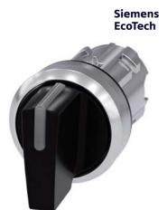
Illuminable selector switch, 22 mm, round, metal shiny, black, Selector switch short, 3 switch positions I>O<II, momentary contact type, actuating angle 2x45°, 10:30h/12h/13:30h
