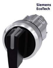
Illuminable selector switch, 22 mm, round, metal shiny, black, Selector switch short, 3 switch positions I-O-II, latching, actuating angle 2x45°, 10:30h/12h/13:30h
