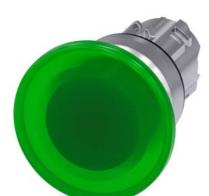
Illuminated mushroom pushbutton, 22 mm, round, metal, shiny, green, 40 mm, momentary contact type, with laser labeling, upper case and lower case, always upper case at the beginning of the word
