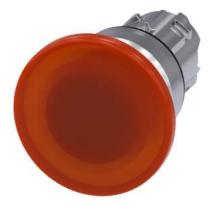
Illuminated mushroom pushbutton, 22 mm, round, metal, shiny, amber, 40 mm, momentary contact type, with laser labeling, lower case  $\,$
