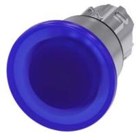
Illuminated mushroom pushbutton, 22 mm, round, metal, shiny, blue, 40 mm, latching, pull-to-unlatch mechanism, with laser labeling, upper case
