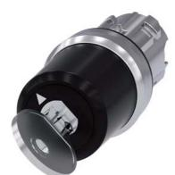
Key-operated switch BKS, 22 mm, round, metal, shiny, lock number S1, with 2 keys, 2 switch positions O-I, latching, actuating angle 90°, 10:30h/13:30h, key removal O, with laser labeling, upper case and lower case, always upper case at the beginning of the word
