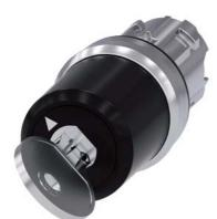
Key-operated switch BKS, 22 mm, round, metal, shiny, lock number S1, with 2 keys, 2 switch positions O-I, latching, actuating angle  $90^{\circ}$ , 10:30h/13:30h, key removal O, with laser labeling, lower case
