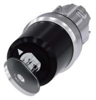
Key-operated switch BKS, 22 mm, round, metal, shiny, lock number S1, with 2 keys, 2 switch positions O<I, momentary contact type, Actuating angle  $45^\circ,$  10:30h/12h, key removal O, with laser labeling, upper case
