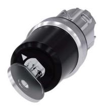
Key-operated switch BKS, 22 mm, round, metal, shiny, special lock, with 2 keys, 2 switch positions O<I, momentary contact type, actuating angle 45°, 10:30h/12h, key removal O, Note: BKS locking systems E1 - E25 supplied without key
