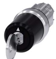
key-operated switch Siemens, 22 mm, round, metal, shiny, lock number SSG10, with 2 keys, 3 switch positions I>O<II, momentary contact on the left, latching on the right, actuating angle 2x45°, 10:30h/12h/13:30h, key removal II, Z=50-unit packaging
