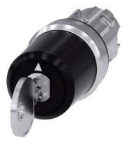
key-operated switch Siemens, 22 mm, round, metal, shiny, lock number SSG10, with 2 keys, 3 switch positions I-O-II, latching, actuating angle 2x45°, 10:30h/12h/13:30h, key removal I+II, with laser labeling, upper case and lower case, always upper case at beginning of line
