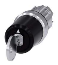
key-operated switch Siemens, 22 mm, round, metal, shiny, special lock, with 2 keys, 3 switch positions I-O-II, latching, actuating angle 2x45°, 10:30h/12h/13:30h, key removal I+II
