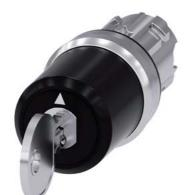
key-operated switch Siemens, 22 mm, round, metal, shiny, lock number SSG10, with 2 keys, 3 switch positions I-O-II, latching, actuating angle 2x45°, 10:30h/12h/13:30h, key removal O, with laser labeling, inscription or symbol customer-specific selection with SIRIUS ACT configurator (CIN)
