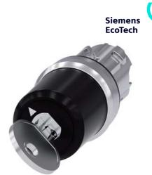
key-operated switch Siemens, 22 mm, round, metal, shiny, lock number SSG10, with 2 keys, 2 switch positions O-I, latching, actuating angle 90°, 10:30h/13:30h, key removal O+I
