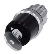
key-operated switch Siemens, 22 mm, round, metal, shiny, lock number SSG10, with 2 keys, 2 switch positions O-I, latching, actuating angle 90°, 10:30h/13:30h, key removal O, with laser labeling, upper case and lower case, always upper case at beginning of line
