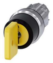
Key-operated switch O.M.R, 22 mm, round, metal, shiny, lock number 73033, yellow, with 2 keys, 3 switch positions I>O<II, momentary contact on the left, latching on the right, actuating angle 2x45°, 10:30h/12h/13:30h, Key removal II, with laser labeling, inscription or symbol Customer-specific selection with SIRIUS ACT configurator (CIN)
